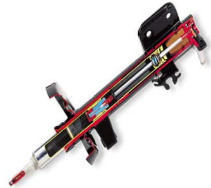
Figure 2: MR fluid based MagneRide shock absorber
